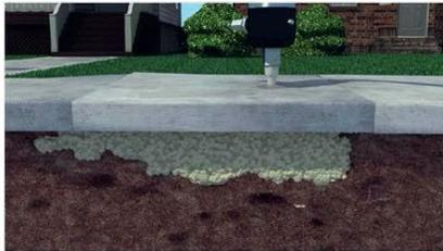
Foam finds low spots and expands in all directions. After approximately six seconds a reaction occurs, expanding into weak soils, compacting, consolidating and increasing density. The foam will expand completely in approximately 15 seconds.
